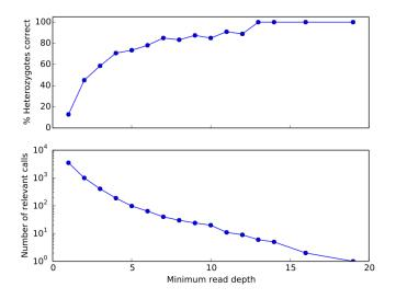
Figure 2-9: Influence of read depth on the accuracy of lobSTR genotypes for heterozygous sites in the Marshfield panel. The fraction of heterozygous individuals correctly genotyped increases monotonically with the minimum number of spanning reads.
