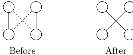
Figure 2-3: Degree-preserving rewiring. Random pairs of non-incident edges are chosen (as shown). If the solid edges are present and the dotted edges are not, these four nodes may be rewired by removing the solid edges and adding the dotted ones.
